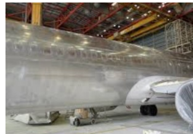
Aircraft masking for paint stripping
